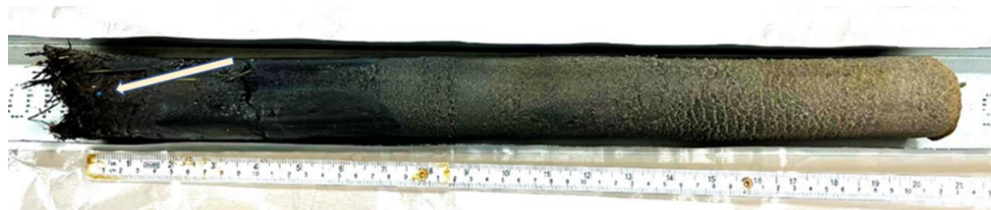
Figure S1. Core 5 sediment core, 52 cm depth. The organic sediment surface on the left contains visible (blue) microplastics. The sandy sediment at lower depths is on the right.
