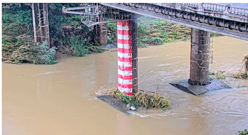
Figure 1. It is challenging to recognize unclear numerical readings in river gauge images. Source: https://fmg.wra.gov.tw/fmgp/ccd_proxy?sn=55 (accessed on 17 October 2022).
