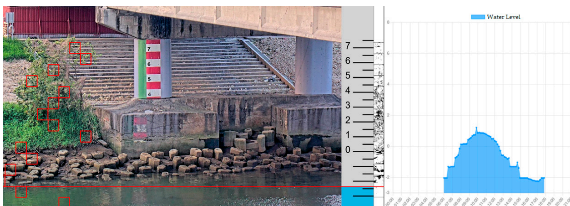
Figure A1. The results of the Water Level Calculation Model. Sunny, 13 April 2022, 6:00 a.m. to 6:00 p.m. The red squares are the grids constituting the virtual water gauge.
