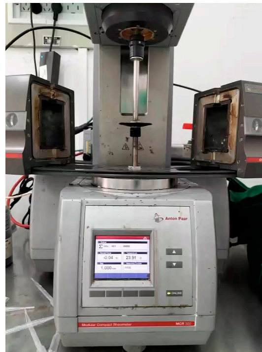
Figure 2. Anton Paar MCR302 Rotational Rheometer.
