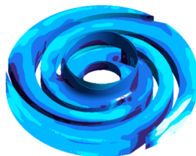
Figure 7. y^+ distribution in impeller fluid domain.
