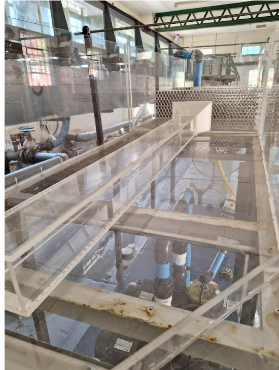
Figure 6. Culvert model from downstream side.
