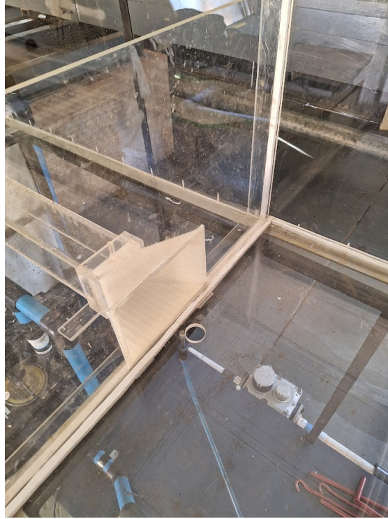
Figure 8. Culvert model with 3D-printed inlet.
