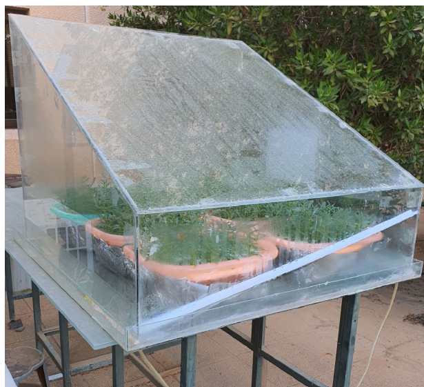
Figure 1. The phytodesalinator used in the phytodesalination experiment with S. portulacastrum plants inside.
