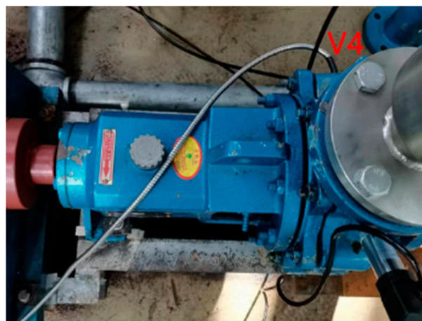
Figure 9. Pressure pulsation monitoring point of the experimental apparatus.
