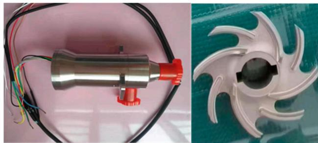
Figure 5. The whole high-speed centrifugal pump and the fully open impeller.
