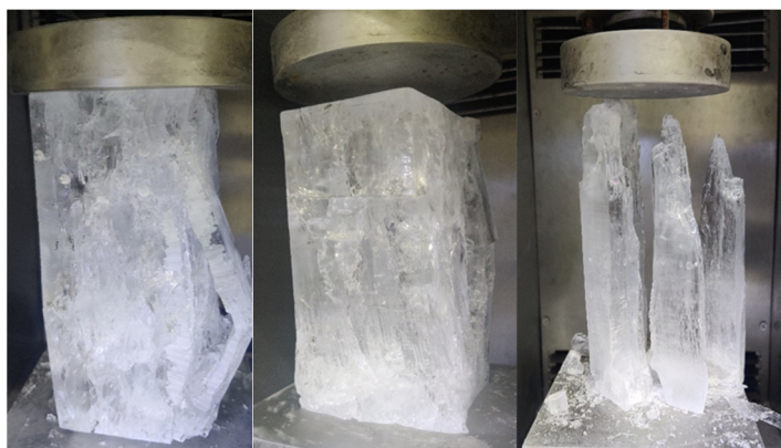
Figure 11. Different types of failure behavior of ice in ductile–brittle transition regime.
