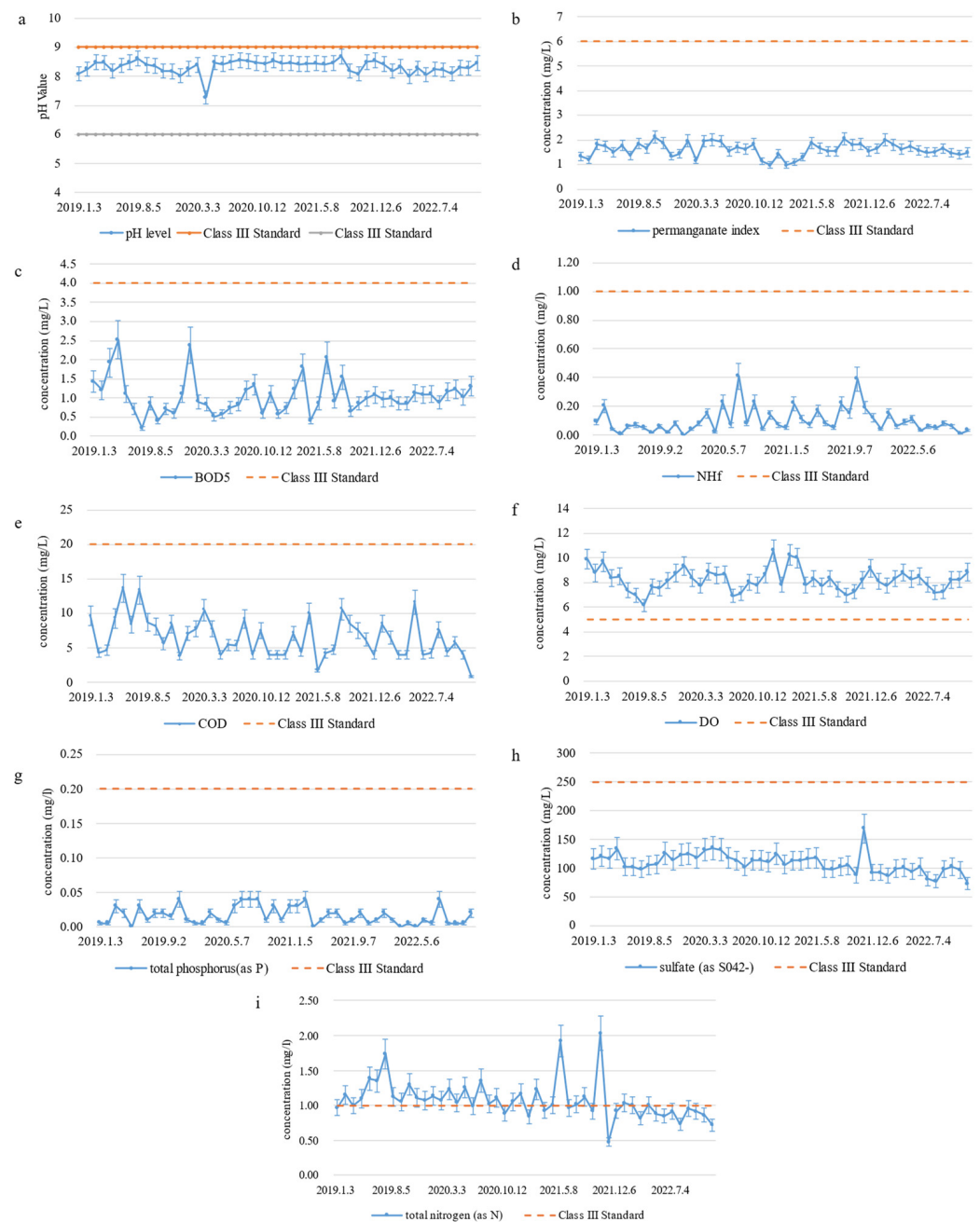
Figure 4. Water-quality trends for (a) pH Values; (b) Permanganate Index; (c) Biochemical Oxygen Demand (BOD 5 ); (d) Ammonia Nitrogen (NH 3 -N); (e) Chemical Oxygen Demand (COD); (f) Dissolved Oxygen (DO); (g) Total Phosphorus; (h) Sulfate (SO 4 2- ); and (i) Total Nitrogen at Zhongzhuang Reservoir.
