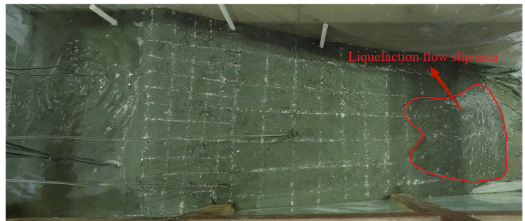
Figure 22. Liquefaction of dam foundation from the top view.
