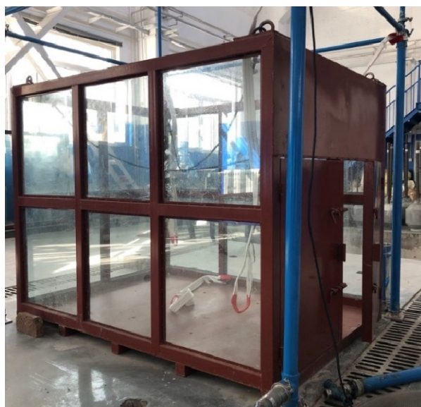
Figure 3. Photo of the model flume.
