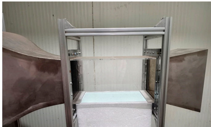
Figure 4. Ice formation tank and test section.
