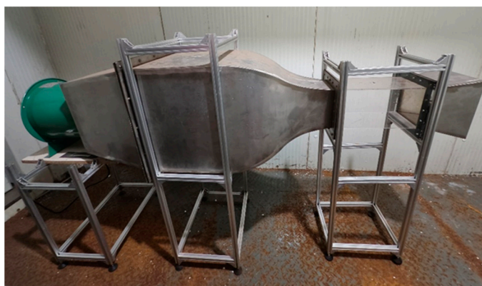
Figure 3. Open-circuit low-speed wind tunnel for this study.
