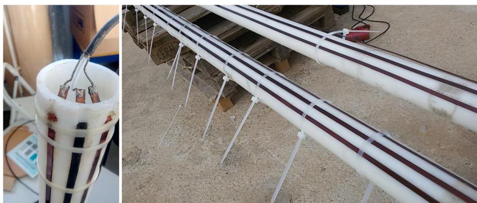
**Figure 6.** The custom TDR probes with three flat enameled copper wires.
