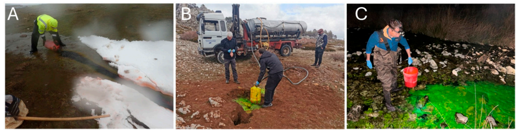
Figure 4. Tracer injection in the tracer tests conducted in Sierra Seca. (A) Eosin in FA hydrogeological basin. (B) Uranine in NAT hydrogeological basin. (C) Uranine in the riverbed of FA River.
