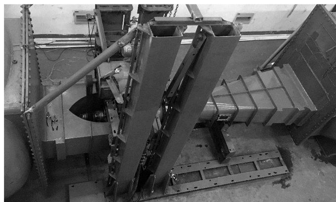
Figure 6. Pumping system model.
