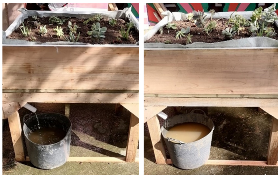
Figure 9. Drainage of the pumice prototype (left) and the expanded clay prototype (right) during the second monitoring session.
