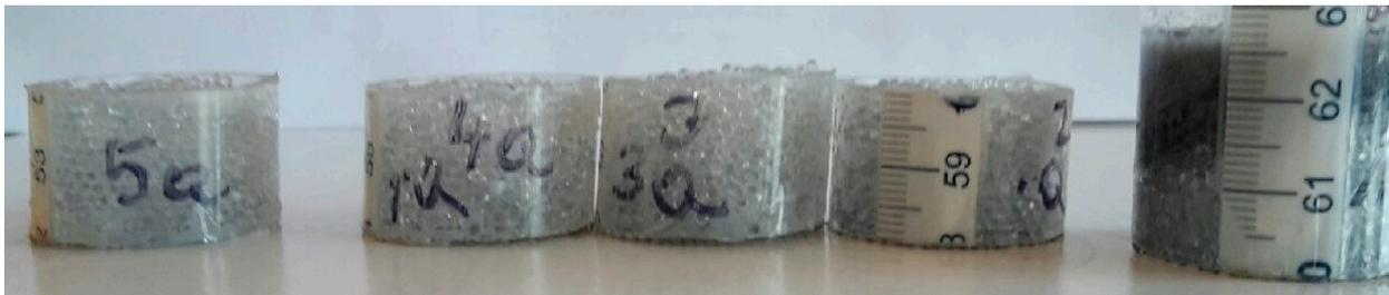
**Figure 5.** The partitioning of columns with accumulated VSSs at different depths. 1a represents the highest filter level (the inlet to the filter), and 5a represents the lowest (the outflow from the filter).
