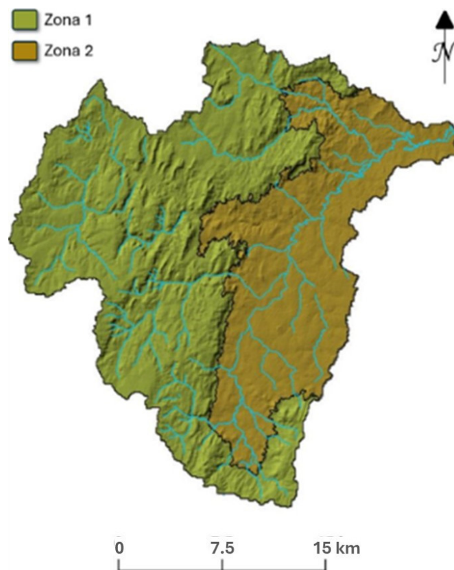
Figure 9. Use of the Terrain Segmentation tool in SAGA GIS (QGIS) to obtain the parameter P (slope) in the APLIS recharge method. The image highlights the geomorphological difference between the Vieira River plain and other drainage areas, most of which are in karst environments.
