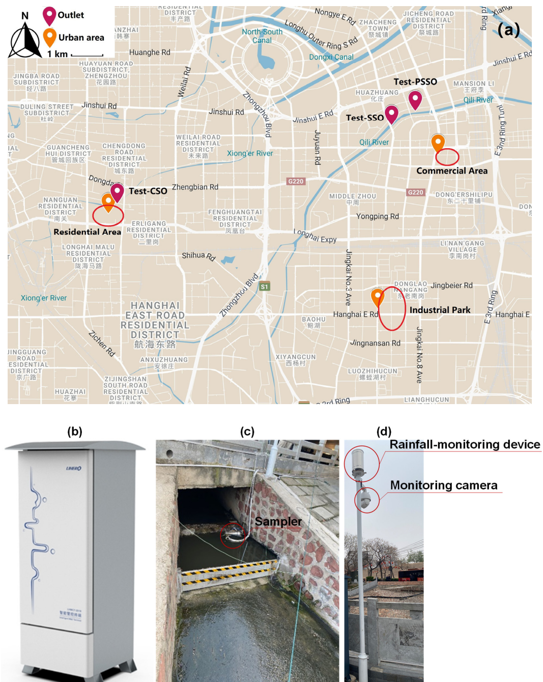
Figure 1. The positional information of the sewer outlets and the equipment for the sampling. (a) Study area (data from the Google Map); (b) autosampler; (c) sewer outlet; (d) rainfall monitoring device.
