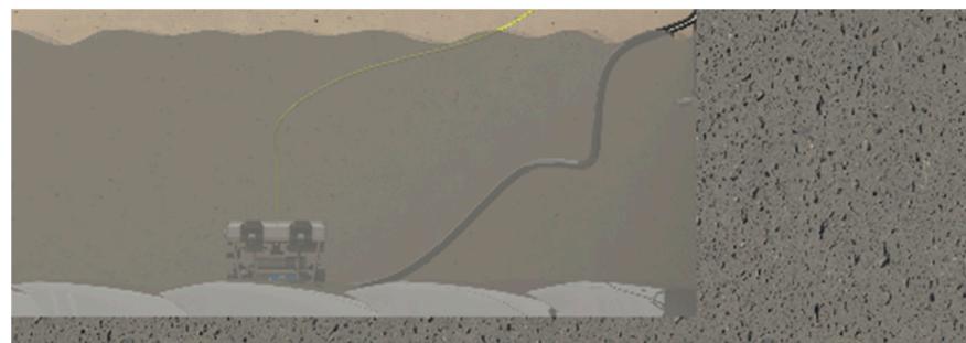
Figure 6. The bottom-sitting dredging operation of the non-aeration section.
