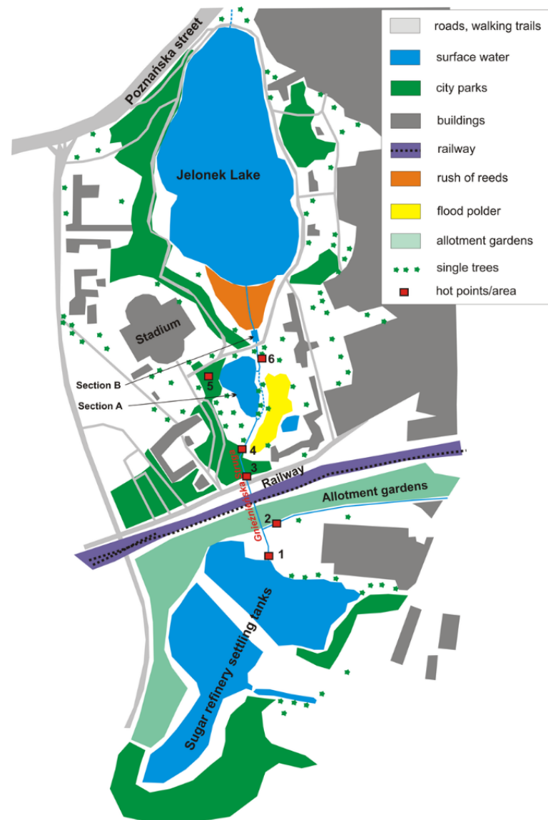
Figure 15. Places of greatest anthropogenic pressure modifying the quality of water in the Gnieźnieńska Struga river: 1—settling tanks of the former sugar factory; 2—allotment gardens; 3—storm sewage system with periodic discharge of municipal sewage from the treatment plant; 4—combined sewage system; 5—temporarily activated storm sewage system; and 6—surface runoff.
