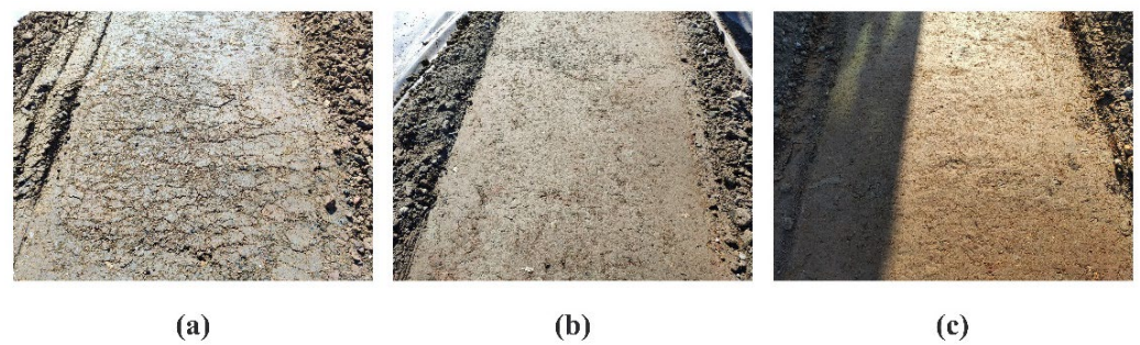
Figure 5. Visual appearance after compaction of dewatered sludge: (a) solidifying agent addition ratio of 0%; (b) solidifying agent addition ratio of 5%; (c) solidifying agent addition ratio of 7.5%.
