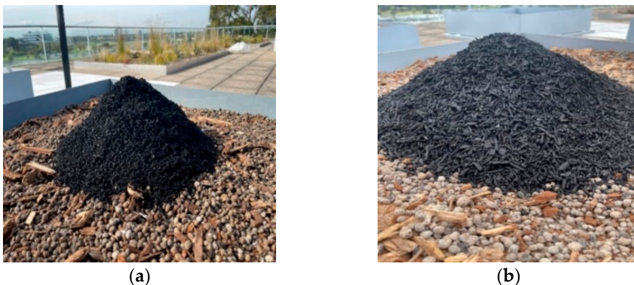
Figure 3. Biochar: (a) Fine particles (less than 1 mm), (b) Medium particles (1–3 mm).
