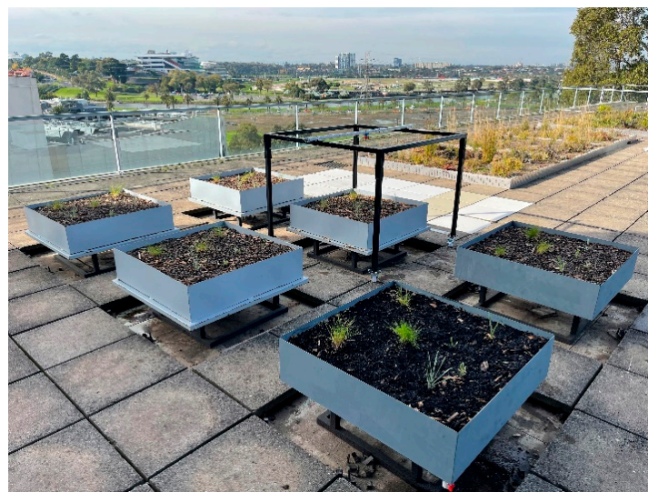
Figure 2. The six 1 m × 1 m green roof test beds on top of Building M at Victoria University, Footscray Park Campus.
