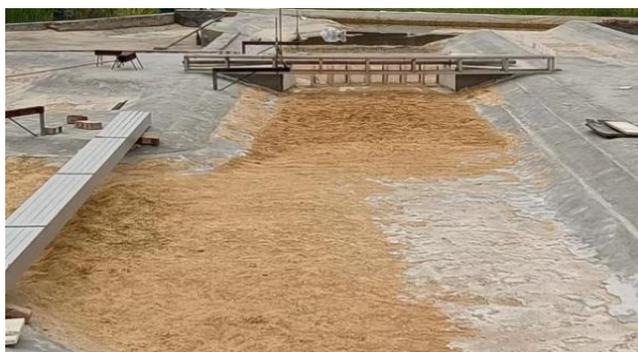
**Figure 14.** Sedimentation distribution in the intersection area after scouring.
