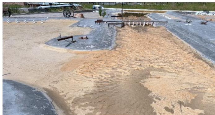
Figure 10. Topographic distribution after the siltation experiment.
