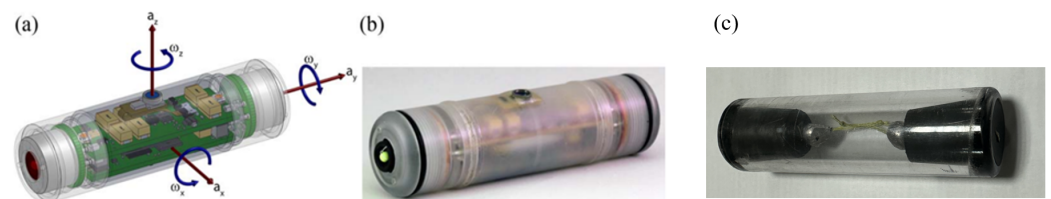
Figure 5. (a) A CAD model of the Sensor Fish and (b) a photo of the Sensor Fish, taken from Deng et al. [14]. (c) A surrogate sensor fish was also fabricated and released during the preparation phase for deployments (see Section 3.3).
