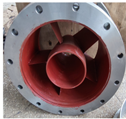
(b) Guide Vane Model
