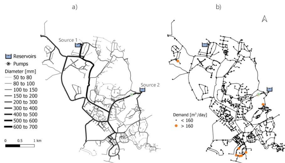
**Figure 2.** Schematic representation of the water distribution network: (a) pipe diameters and (b) location of large consumers.
