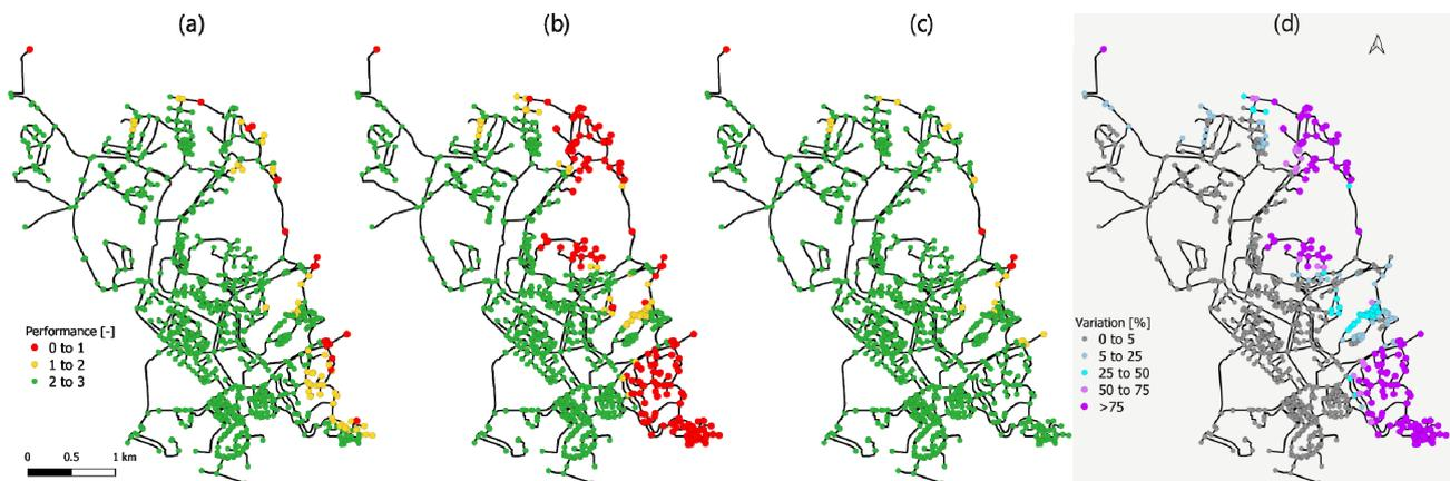
**Figure 8.** Spatial distribution of the minimum pressure index for year 20, at the peak-hour consumption (2 h): (a) Reference scenario; (b) Scenario 1 (demand increase and older pipes); (c) Scenario 2 (demand decrease and renewed pipes); and (d) Relative variation from Scenario 1 and Scenario 2 relative to the reference scenario.
