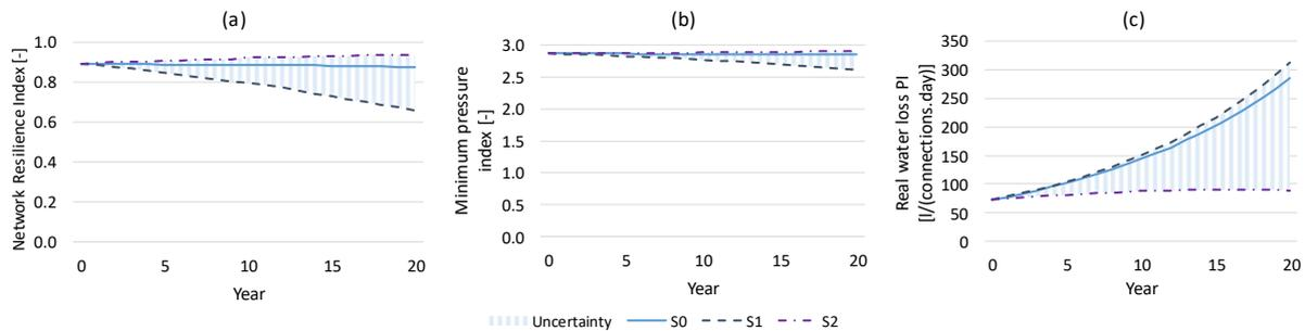
**Figure 9.** Evolution of the performance assessment metrics for the different scenarios: (a) network resilience index; (b) minimum pressure index; and (c) real water loss performance indicator.
