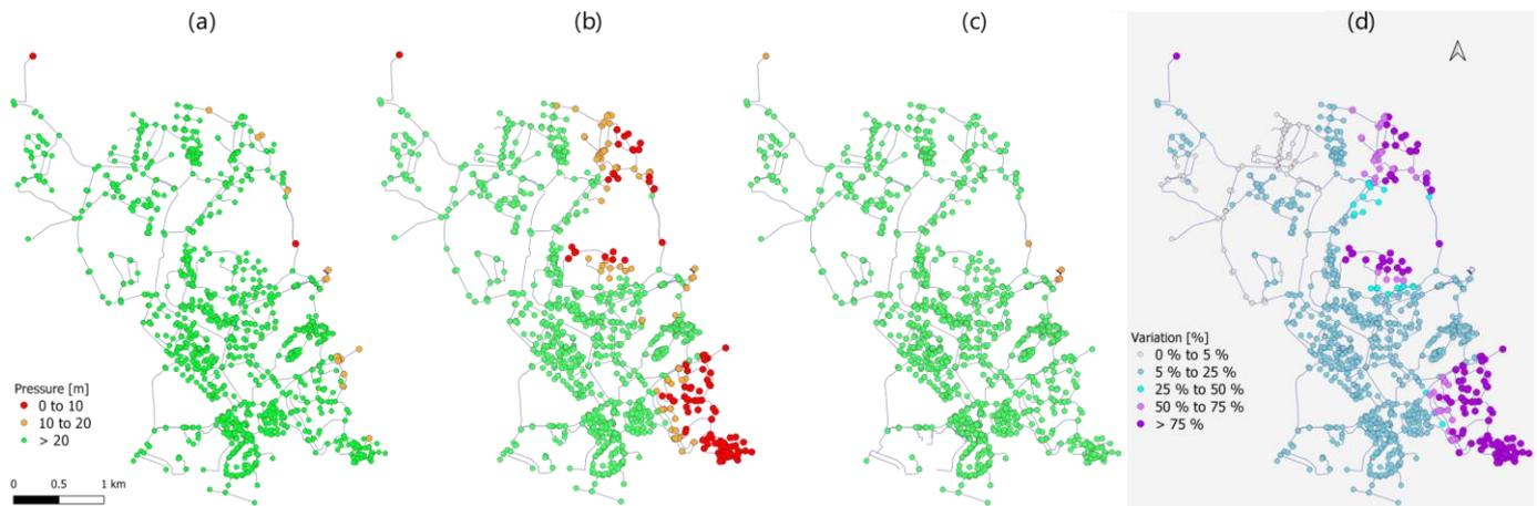
**Figure 6.** Spatial distribution of minimum pressures in nodes for year 20, at the peak-hour consumption (2 h): (a) Reference scenario; (b) Scenario 1 (demand increase and low rehabilitation rate); (c) Scenario 2 (demand decrease and adequate rehabilitation rate); and (d) Relative variation from Scenario 1 and Scenario 2 with respect to the reference scenario.
