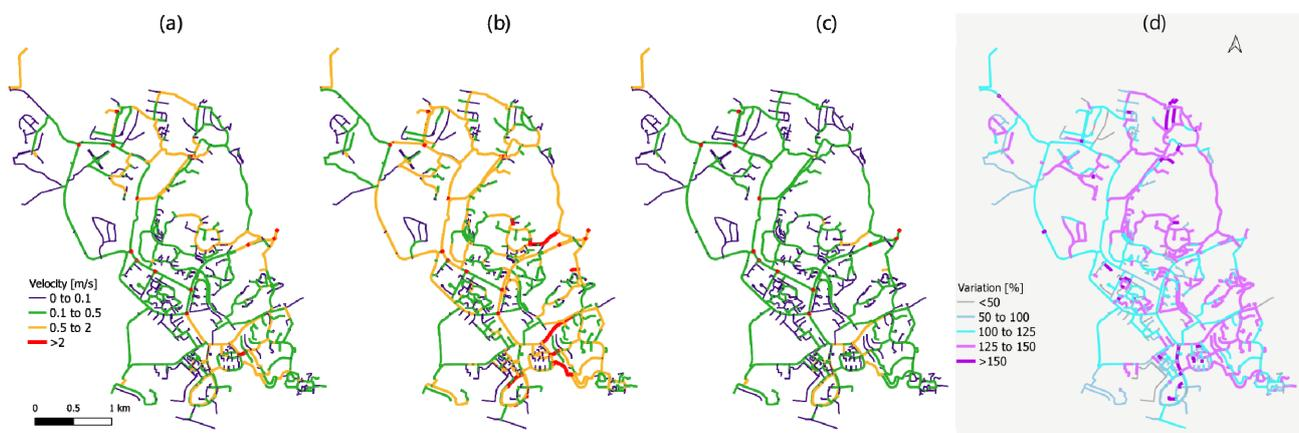
**Figure 7.** Spatial distribution of maximum velocities in pipes for year 20 at the peak-hour consumption (2 h): (a) Reference scenario; (b) Scenario 1 (demand increase and low rehabilitation rate); (c) Scenario 2 (demand decrease and adequate rehabilitation rate); and (d) Relative variation from Scenario 1 and Scenario 2 with respect to the reference scenario.
