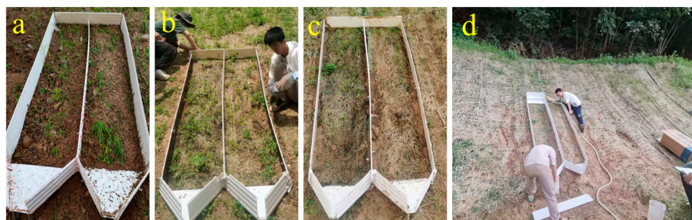
Figure 2. Schematic diagram of runoff plot. (a) Unrepaired slope plot, (b) repaired filled slope plot, (c) repaired excavated slope plot, (d) erosion process.
