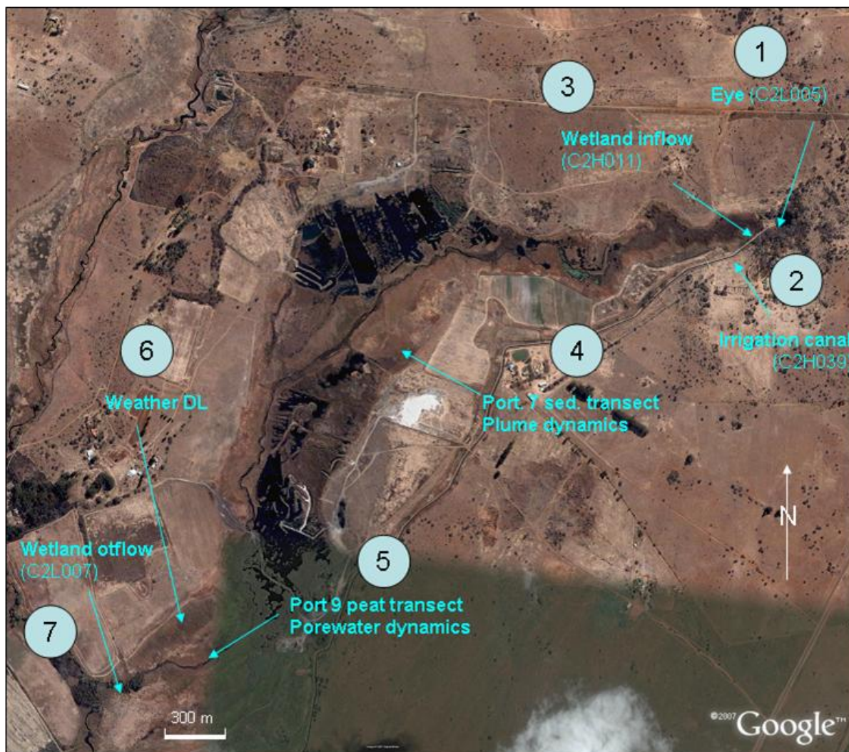
Figure 12. Location of automatic measuring stations installed in the Gerhard Minnebron Wetland (DL-data logger).
