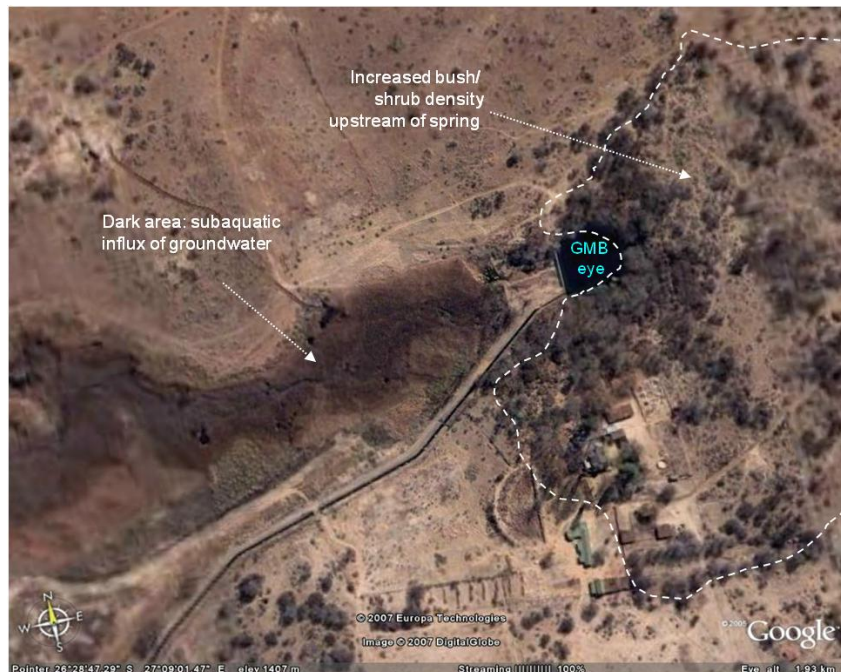
Figure 6. A satellite image of the Gerhard Minnebron wetland taken during winter depicting an increased bush/shrub density towards the eye as point where the increasingly shallower groundwater table finally intersects the topographic surface as well as darker areas within the downstream wetland. Both features have been found at other sites in the region to indicate shallower groundwater levels and exfiltrating conditions, respectively (Satellite image: Google Earth, 2008).
