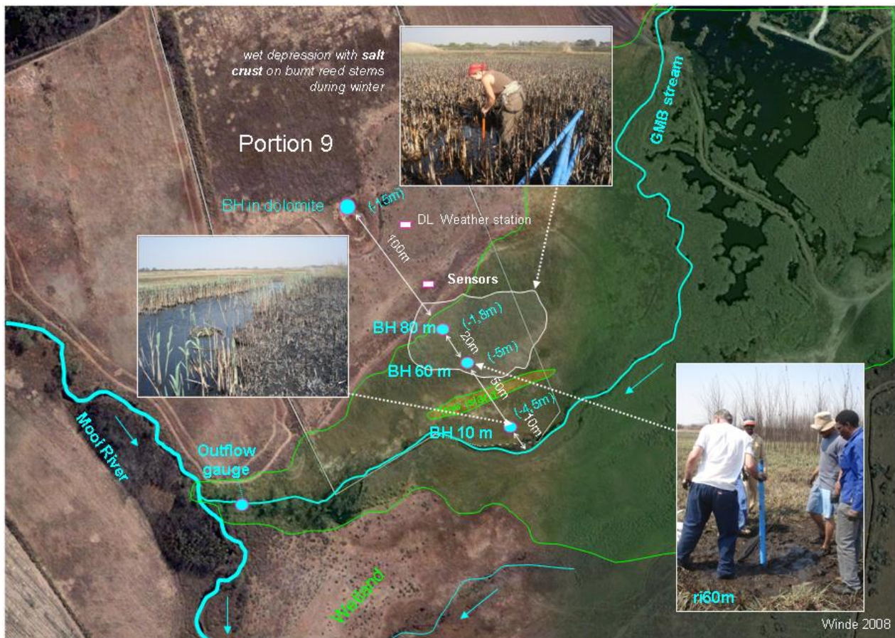
Figure 18. Location and structure of the borehole transect in peat installed at portion 9 (underlying satellite image retrieved from Google map, September 2008).
