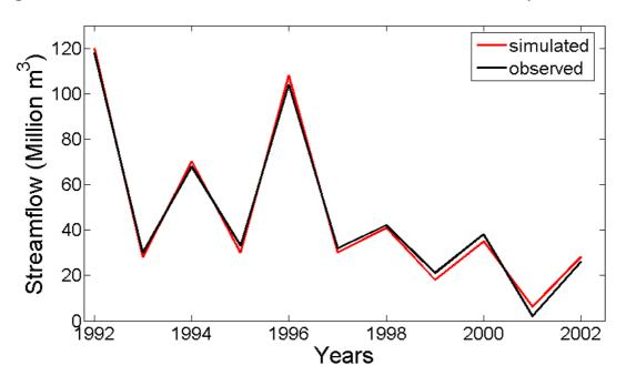
Figure 3. Observed and WEAP simulated streamflow time series at Rheraya catchment.
