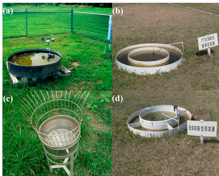
Figure 1. Four types of evaporation evaporimeters: Class A from the USA (a); GGI-3000 from Russia (b); and \phi 20 (c) and E601B (d) from China.
