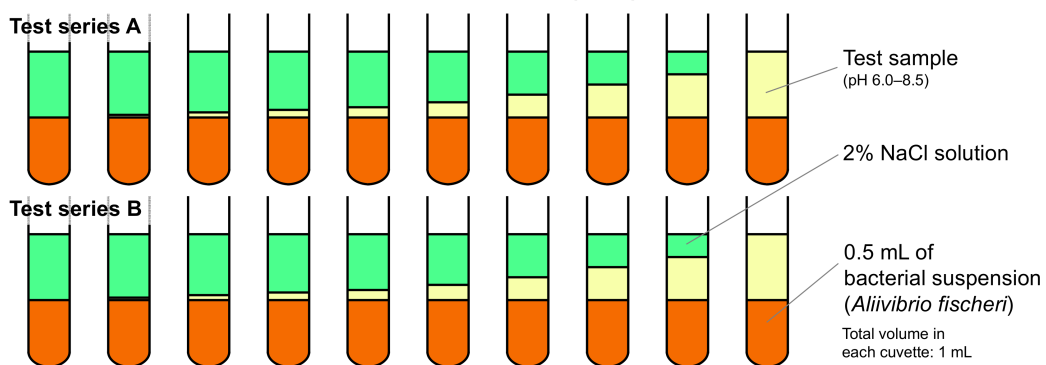
Figure 1. Construction of the bacterial inhibition tests used in this work (ATU: N -allylthiourea).
