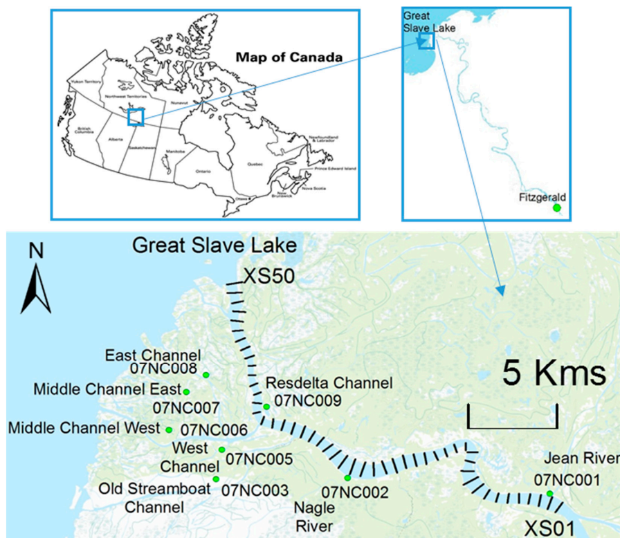
Figure 1. The Slave River Delta with important channels. (The dark lines in the bottom panel represent cross-sections spaced 500 m apart. Widths of cross-sections vary between 500 and 1200 m).
