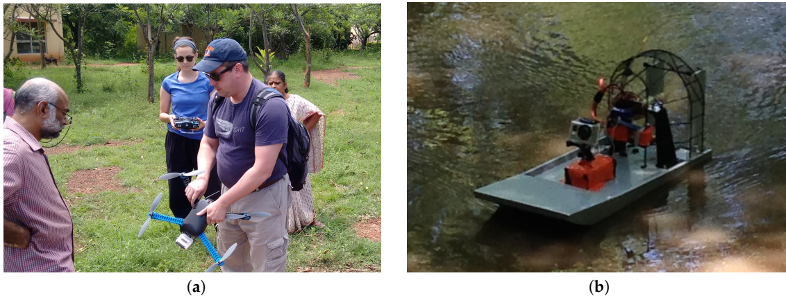
Figure 4. (a) Demonstrating the 3DR Iris quadcopter near Bangalore (note: the sensor shown here mounted to the UAV is different from the Sony ActionCam used for data acquisition); (b) The custom USV airboat used for bathymetric data collection in the Arkavathy Basin.
