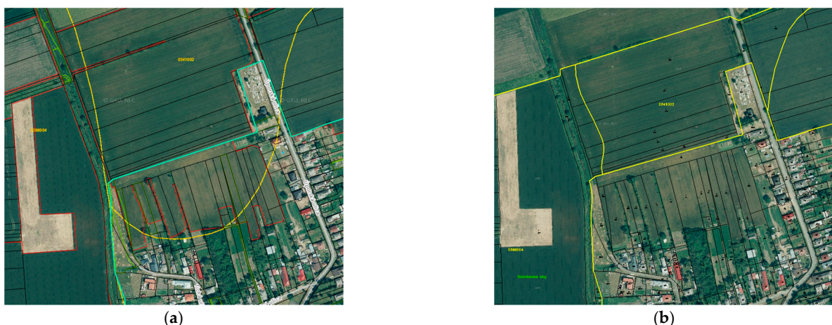
Figure 17. Illustration of differences in the registration of EPEU areas in the cadastral unit after LC registration into the real estate cadastre: (a) Agro layer of ZBGIS; (b) from the real estate cadastre.
