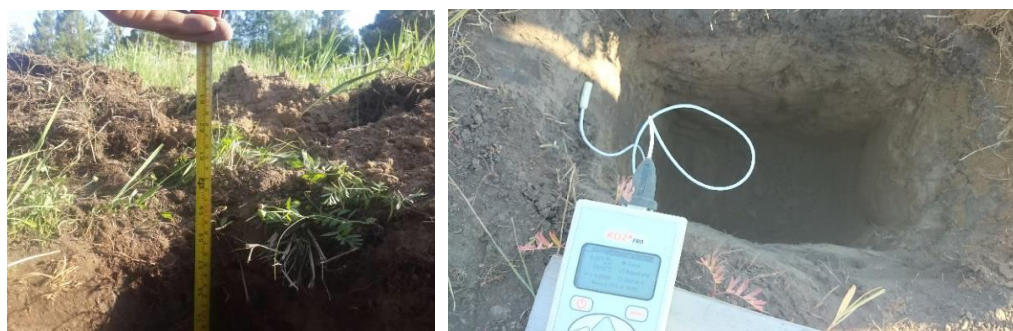
Figure 12. Soil sampling and in-situ measurements of thermal properties (thermal conductivity, thermal diffusivity and volumetric heat capacity) using a KD2 Pro needle probe.
