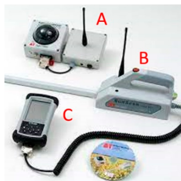
Figure 2. Main components of the SunScan system: (A) Dome sensor; (B) Probe; (C) Field computer.
