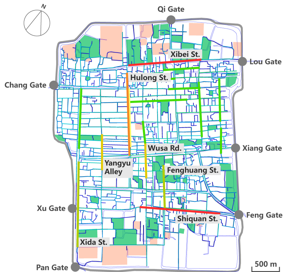
Figure 3. Street axis model analysis results. Streets marked in red are the most integrated streets, and those marked in dark blue are the least integrated streets. Streets with a higher degree of integration have more intersections with other streets, and streets with a lower degree of integration have fewer intersections with other streets.
