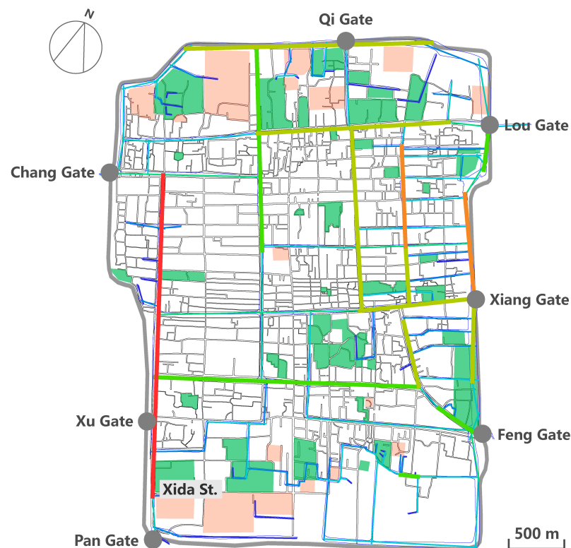
Figure 5. Canal axis model analysis results. Canals marked in red are the most integrated canals, and those marked in dark blue are the least integrated canals. Canals with a higher degree of integration have more intersections with other canals, and canals with a lower degree of integration have fewer intersections with other canals.
