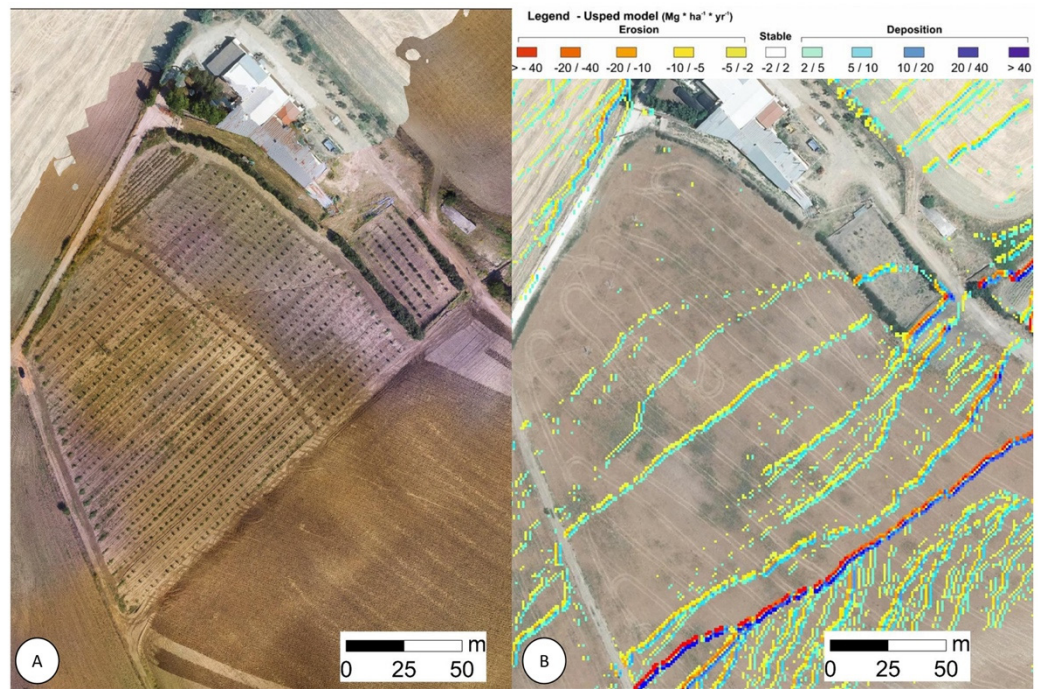
Figure 8. Details of the cultivated hazelnut area, (A) orthophoto derived from UAV data; (B) erosion map by USPED model.
