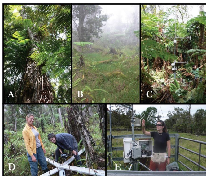
Figure 3. Taking micrometeorological measurements of water fluxes in native forest and pasture in Kona, on the west side of Hawai'i Island, to measure groundwater recharge, the sole source of water for the coastal community [52–54]. (A) Large, complex, and multi-layered leaves within Kahalu'u Forest have high surface area that intercepts fog and contributes to groundwater recharge; (B) Fog interception by leaves is somewhat lower in this more open forest; (C) Kate Brauman setting up a micrometeorological station in forest; (D) Kate Brauman and Heather Tallis setting up devices for measuring the amount of precipitation that falls through the forest to the ground (as opposed to evaporating from leaf surfaces); (E) Kate Brauman taking meteorological measurements on Palani Ranch (PC: Gretchen C. Daily, A–E).
