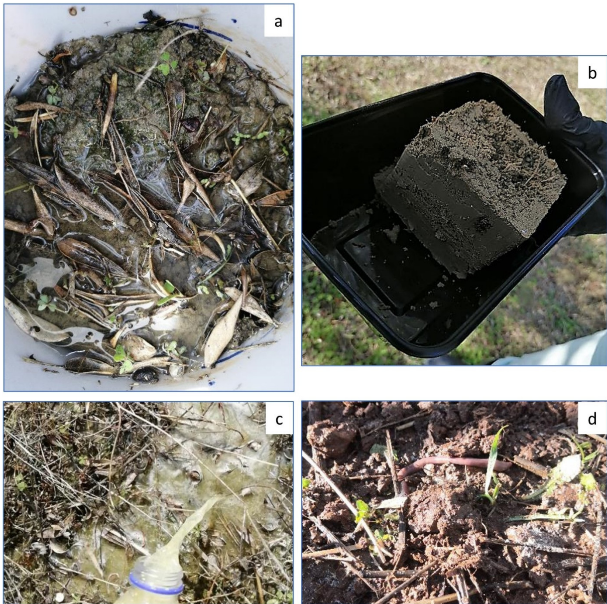
Figure 2. (a) Infiltration rate experiment, (b) soil sampling for bulk density measurement, (c) pouring mix of water and mustard for earthworm test in Astrikas, and (d) worms coming out to surface after the pouring of the mix in Alikambos.
