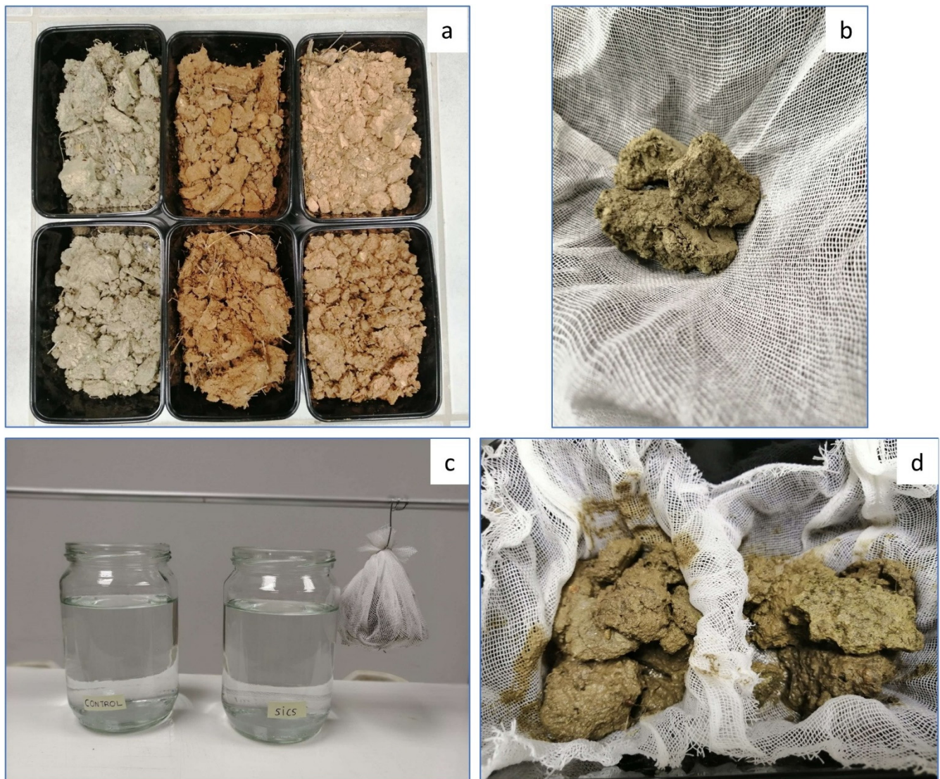
Figure 3. (a) Soil aggregates from both plots (control and SICS) of the three study sites: air-drying before slaking test, (b) 100 g of three aggregates of the Astrikas field to be used for the slaking test, (c) soil aggregates into the mesh before being immersed to water, and (d) soil aggregates after the immerse to water.
