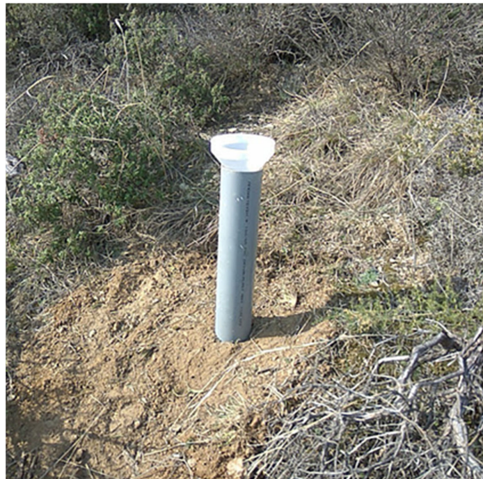
Figure 11. View of the installed cumulative rain gauge in the study area.
