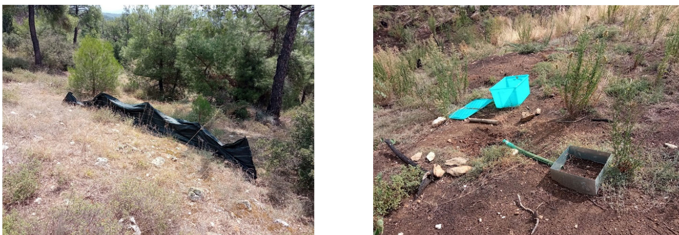
Figure 8. Silt fence which was damaged by humans trying to pullout the metal rebars and geotextile (left). Damage to the experimental setup for the measurement of runoff (right).
