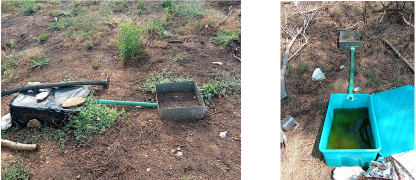
Figure 10. Experimental setup for the measurement of surface runoff (left). Water gathered in the plastic tank after an intense rainfall event (right).
