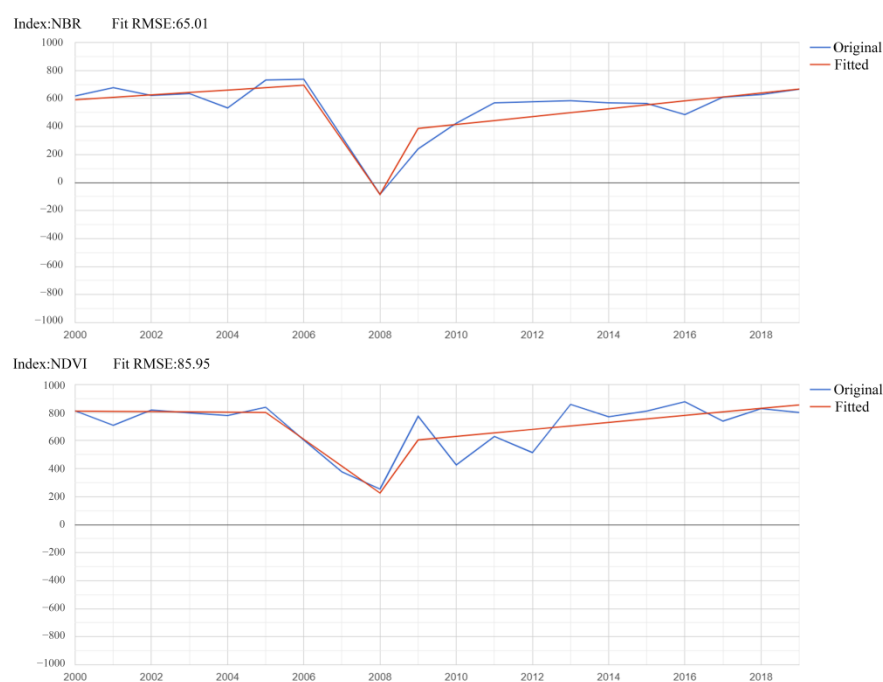
Figure 3. The fitting process of the LandTrendr algorithm. One example of the fitting calculation process. The root mean square error (RMSE) of the final fitting based on NDVI was 85.95 (the actual value should be 0.08595) but the RMSE based on NBR was 65.01 (that is 0.06501), which was slightly lower than that of NDVI.
