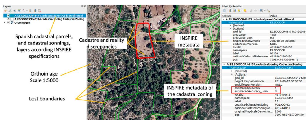
Figure 1. Example of Spanish INSPIRE Cadastral Parcel and Cadastral Zoning layers (themes) information. In the figure, one can see ground lost boundaries and cadastral and reality discrepancies. Source: own elaboration.
