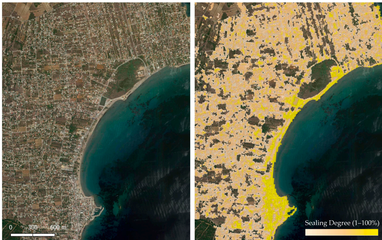
Figure 2. Incorrect classification in the eastern Attica zone (Greece), with the beach area classified as highly sealed impervious area (sealing degree close to 100%).
