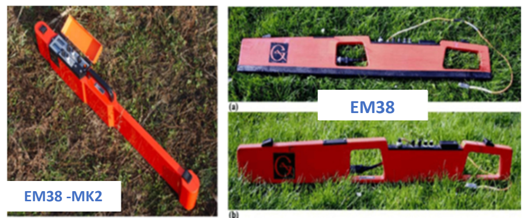
Figure 1. The EM38-MK2 and EM38 devices. (a) The EM38 in horizontal mode. (b) The EM38 in vertical mode (from Geonics Ltd., Catalano [37] and Siddique [38]).
