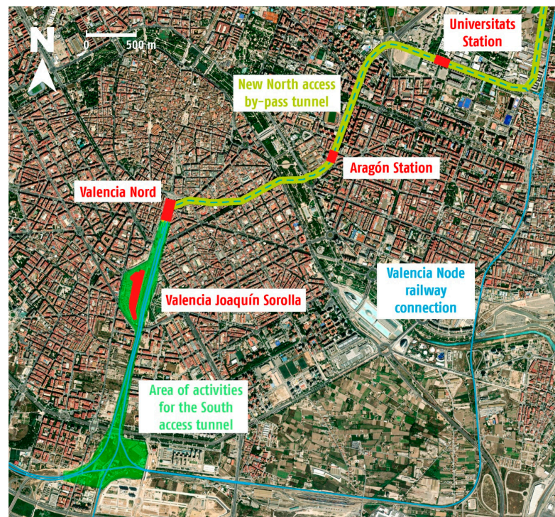
Figure 7. Functional diagram of the Parc Central and Access Canal project, with through-tunnel and new north station (Aragón). Source: ADIF.
