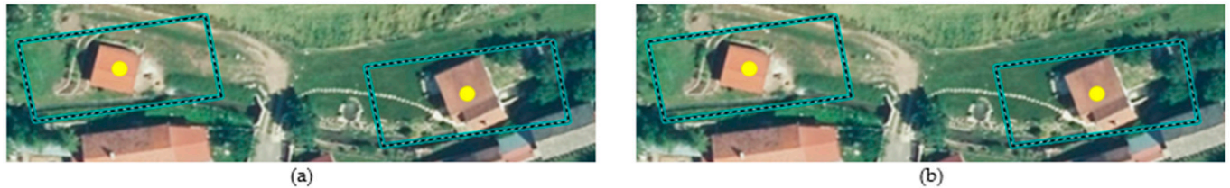
Figure 12. Example of the verification process based on data from the dataset Sentinel-2 L2A—True color: (a) 2017 dataset on the orthophoto base map 2018; (b) 2018 dataset on the orthophoto base map 2018.
