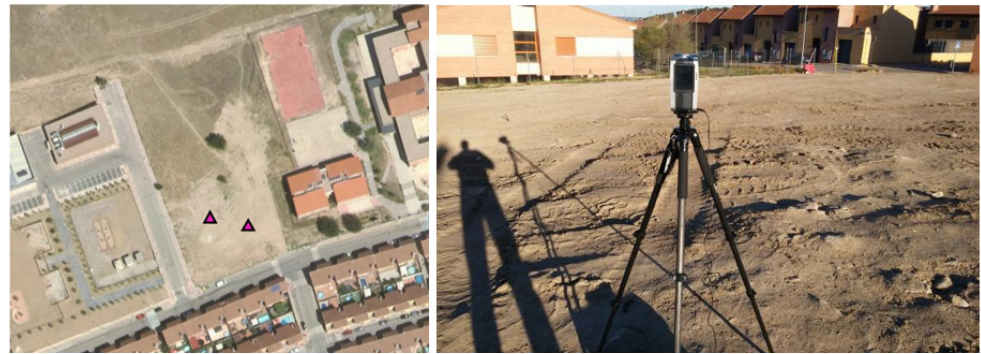
Figure 2. Positions (marked with the triangles) of the LIDAR measuring stations in the plot (left), and detail of the LIDAR (right).
