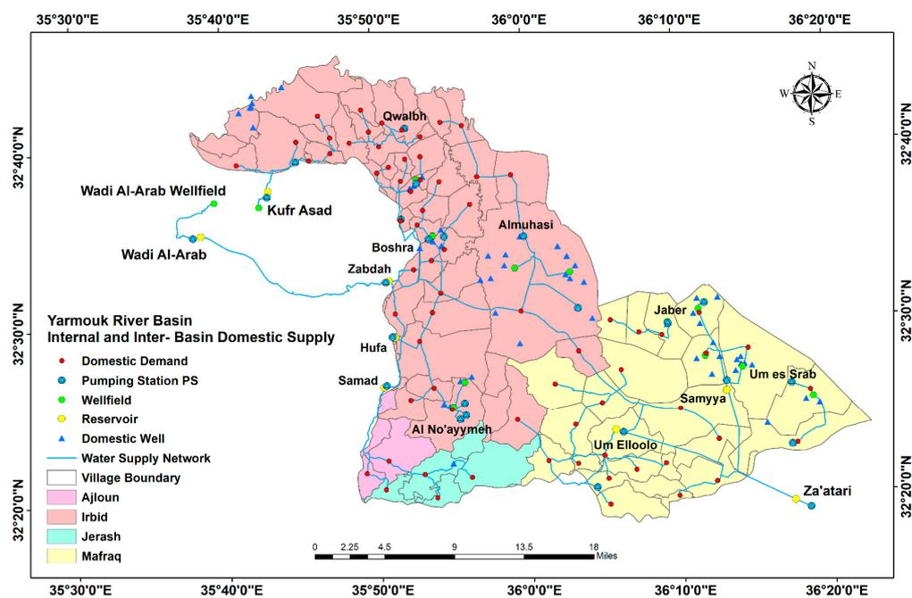
**Figure 4.** Internal and inter-basin domestic water supply for the Yarmouk River Basin.
