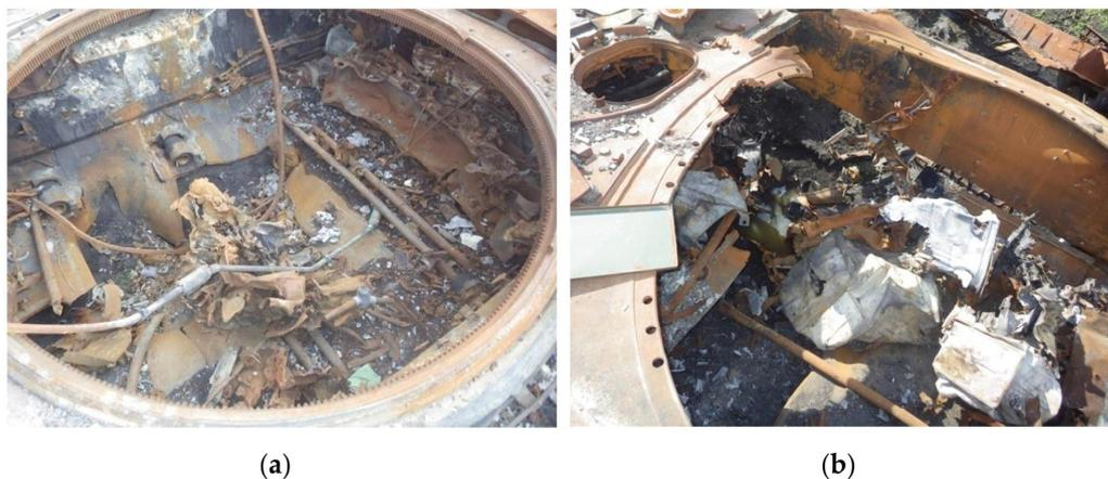
**Figure 2.** Images of the damaged transport-loading vehicles: detonated T-72 tank (a) after the explosion of the ammunition in the middle of the tank (where the ammunition was stored); (b) detonated front part of a T-80 tank (the ruptured right side of the tank, near the place where the driver sits).
