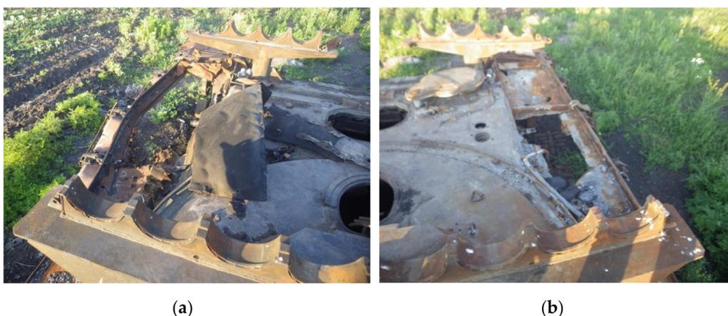
**Figure 3.** Images of the damaged transport-loading vehicles: the points of impact on the TOS-1 “Solntsepek” on the upper part of the hull on the left (a) and right (b) sides (the fuel tanks).
